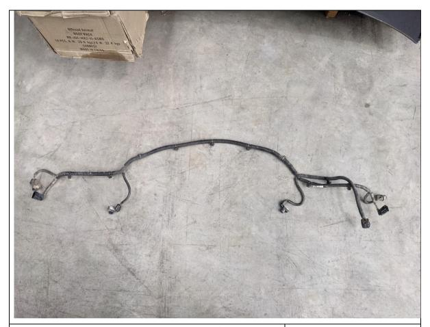
12. Remove the main rear bar wiring harness (with parking sensors attached) from the bumper, by unclipping harness connections with a trim tool.
